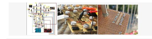
Getting the electronics right in this project is by fare the hardest task in this project. If you can make a PCB, go for it, as it will save a lot of time fixing minor errors. Otherwise, use a stripboard, as you won't need any special tools. You can follow the wiring as shown in the Fritzing file found in **Acoustic Meeblip Scheme.zip**.
