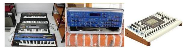
FIGURE 7. THREE COMMON FORM FACTORS FOR SYNTHESIZERS (KEYBOARD, RACK-UNIT, TABLETOP)
