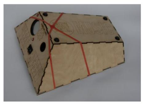
FIGURE 45. HOW A RUBBER BAND HOLD THE DEVICE TOGETHER
